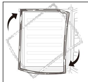
8. Place the door back on. Ensure the door is aligned
