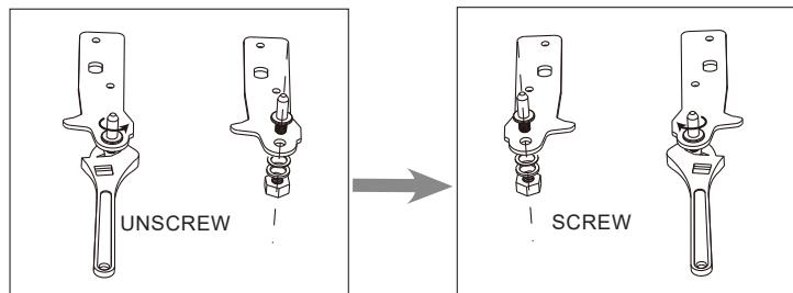
6. Refit the bracket fitting the bottom hinge pin.
