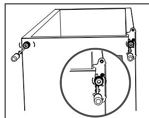
5. Unscrew and remove the bottom hinge pin, turn the bracket over and replace it.
