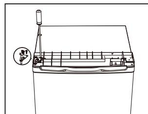
9. Put the top cover and fix it with 2 screws on the back.
