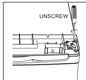
4. Unscrew bottom hinge of freezer door. Then remove the door and place it on a soft pad to avoid scratch.
