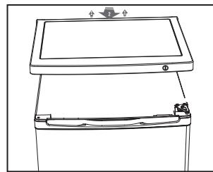
3. Unscrew top hinge and then remove door and place it on a soft pad to avoid scratch.
