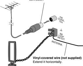
AM loop antenna Keep it connected.
