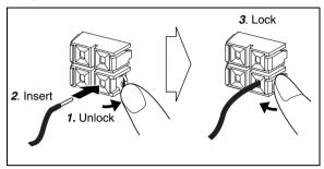
When connecting the speaker cords, match the polarity of the speaker terminals: The black cord to (–), the red cord to (+).
