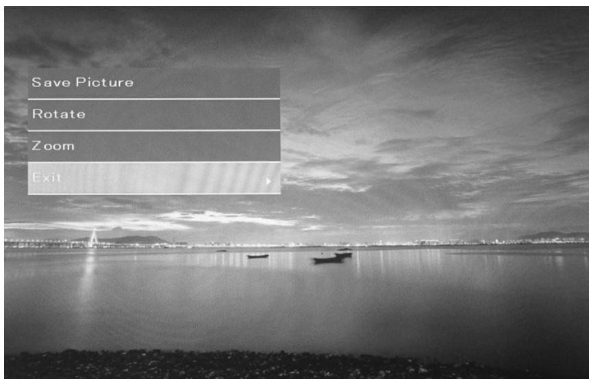
Select Save picture and then press the **>||** key to save the photo into built-in memory. Unit with built-in 8M memory, it can load maximum 5 images with 480\*234 resolution, supports max JPEG file size 64M (8000\*8000).
