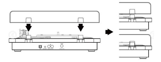
Note: Take care when fitting, and do not press down too hard. Remove the dust cover in the same manner, but pull the cover upwards.
