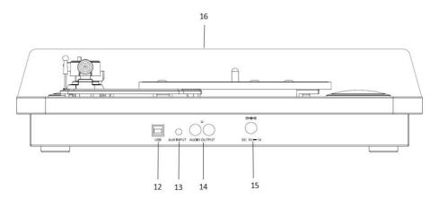
12. **USB Audio Output** - Use the included USB cable to connect your turntable to your computer. The USB connection will send audio from the turntable to your computer.
