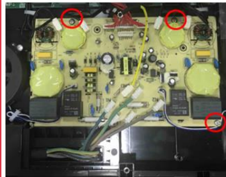
Accessorial power board
