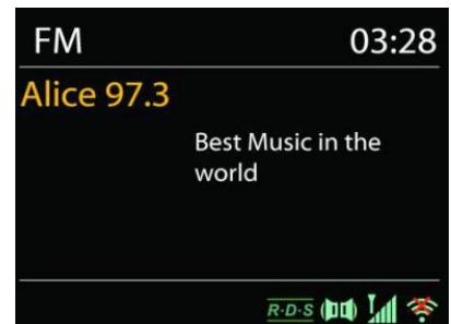
To full scan, press “INTRO” remote key. The frequency display starts to run and scans the FM full band.
