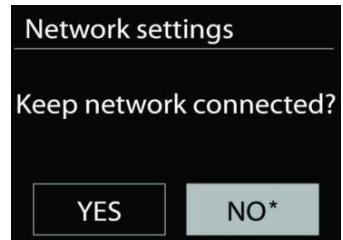
When Keep network connected is selected the standby power consumption is raised.
