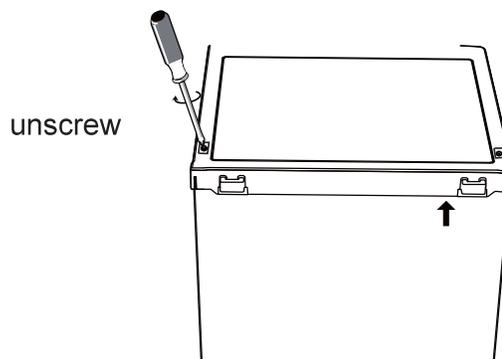
2. Carefully lift the top cover 5CM away from the freezer, then pull out the terminal. Then remove the top cover away.
