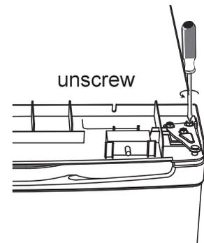
4. Remove the screws and bottom hinge. Then remove the adjustable feet from both sides.
