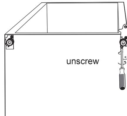
5. Unscrew and remove the bottom hinge pin, turn the bracket over and replace it.
