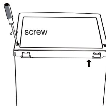
10. With the door closed, check that the door is aligned horizontally and vertically and that the seals are closed on all sides before
