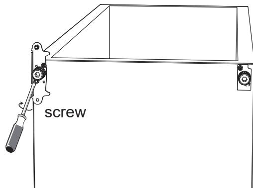
7. Place the door back on. Ensure the door is aligned horizontally and vertically so that the seals are closed on all sides before
