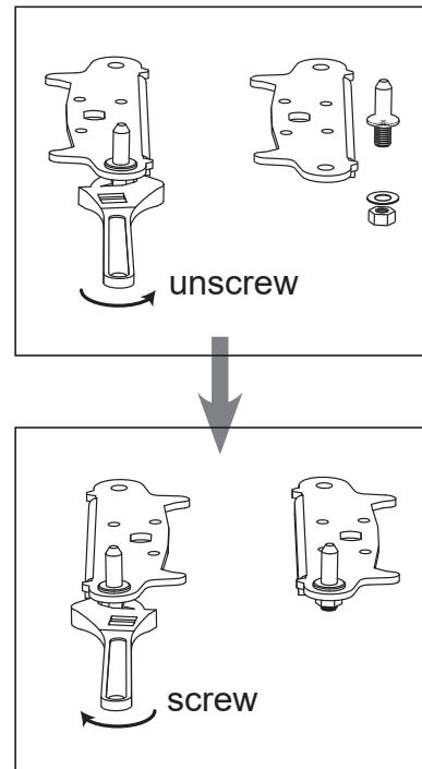
6. Refit the bracket fitting the bottom hinge pin. Replace both adjustable feet.
