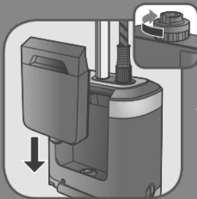
**EN** Fully screw the water tank cap and insert tank back in appliance.
