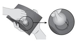
Turn the stand clockwise until it reaches the second groove. When detaching the stand, turn it counterclockwise until it reaches the first groove.
