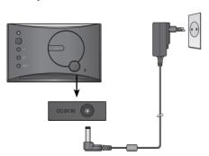
Press the POWER button on the back of the product to turn the power on. When turning off the power, press the POWER button for 2 ~ 3 seconds until the screen goes off.
