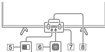
**⑤ BUILT-IN MIC SWITCH\*<sup>5</sup>:** Turn on/off the built-in MIC.
