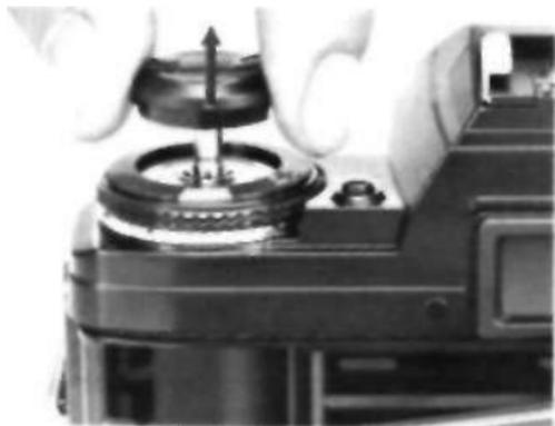
1. With the case off, pull up on the back-cover release knob until the camera back springs open. Gently blow away any dust or other particles inside with a blower brush.
