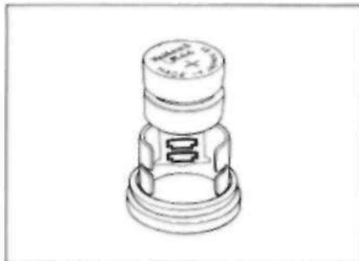
2. After wiping the terminals with a clean, dry cloth, hold the batteries by their edges and insert them plus (+) side out into the sleeve on the inside of the cover.
