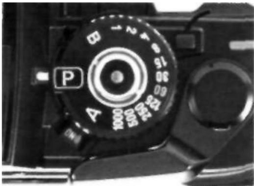
Mode/shutter-speed selector and P/A-lock release
