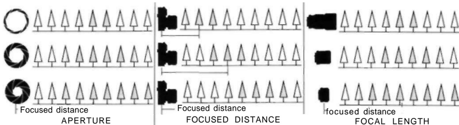
The range behind and in front of the focused distance within which the image appears acceptably sharp is called the depth of field.
