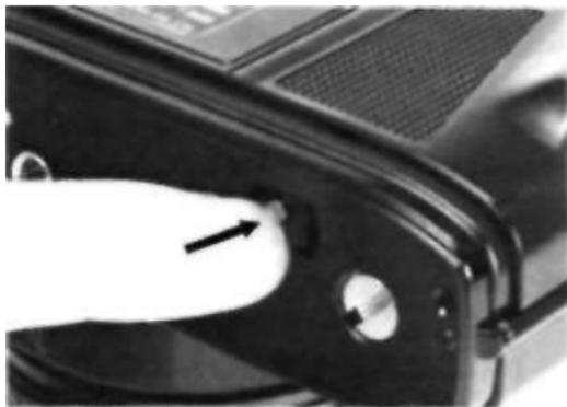
1. To rewind the film, remove the camera's case if on, then press the rewind release on the camera bottom.
