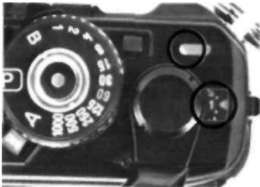
6. Advance film, release shutter, and advance film — until the index points to "1". A red bar should now appear at far left in the Safe Load Signal, indicating film is loaded and advancing properly. (If it does not appear or swings far to the right, repeat steps 3 to 6.) The camera is now ready for taking the first picture, provided film speed is set.
