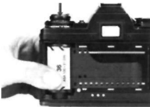
2. Leaving the knob pulled out, position a 35mm film cartridge as shown with the projecting spool facing down. Then push the knob all the way in, rotating it slightly if necessary.
