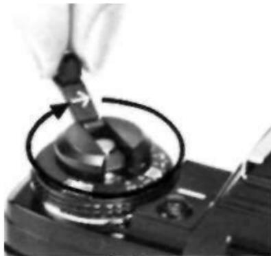
2. Unfold the rewind crank and turn it in the direction of the arrow until the red bar in the Safe Load Signal moves out of the window to the left. Near the end you will feel tension on the film increase then completely disappear, and the crank will then turn freely.
