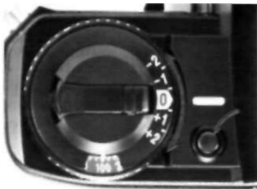
To deliberately increase or decrease exposure from the normal metered value, turn the exposure-adjustment control while pressing the lock release until the desired position is aligned with the index. Set minus (−) numbers to darken exposure and plus (+) numbers to lighten exposure, as indicated in the table.
