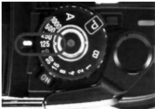
Set mode/shutter-speed selector at any position from " 1 " to "1000".
