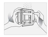
Thoroughly rinse the inside and outside of the strainer under running water.
