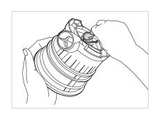
The silicone ring is removable for cleaning. After cleaning, place the silicone ring on as shown in the picture.
