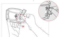
TIP | Insert into the slot with the tail pointing down.
