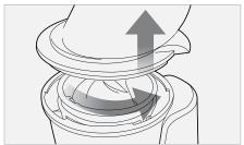
When moving the appliance, do not lift by grabbing the feeding tube. Always lift the appliance by grabbing the base or handle.
