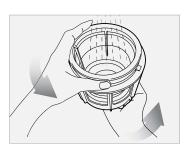
4 After cleaning, remove the strainer from the cleaning tool. Dry before storing.
