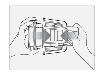
Under running water, rotate the cleaning tool and the strainer in opposite directions to clean.
