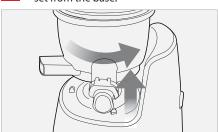
Note | • Immediately clean the juicer after each use by lifting off the drum-set from the base. (Removing the juicing screw and strainer while drum-set is still on the base may cause dripping.)
