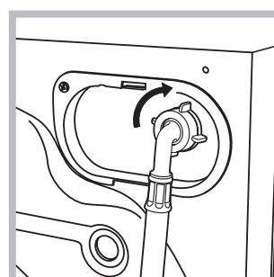
1. Connect the supply pipe by screwing it to a cold water tap using a  $\frac{3}{4}$  gas threaded connection (see figure). Before performing the connection, allow the water to run freely until it is perfectly clear.
