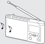
2 Press and hold the desired preset button (1 - 5) until "Station saved to preset x." appears on the display.
